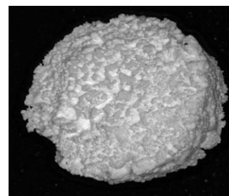
Figure 6. Side image of bound powder after STA analysis.
